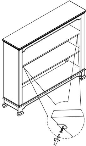
To adjust the shelf, release the screw from the bottom as shown.
