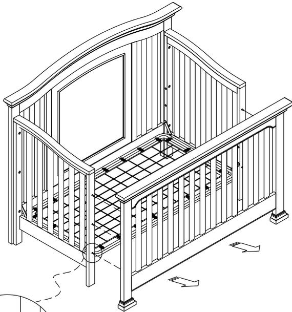
Remove the bolts from the footboard using the allen wrench provided.
