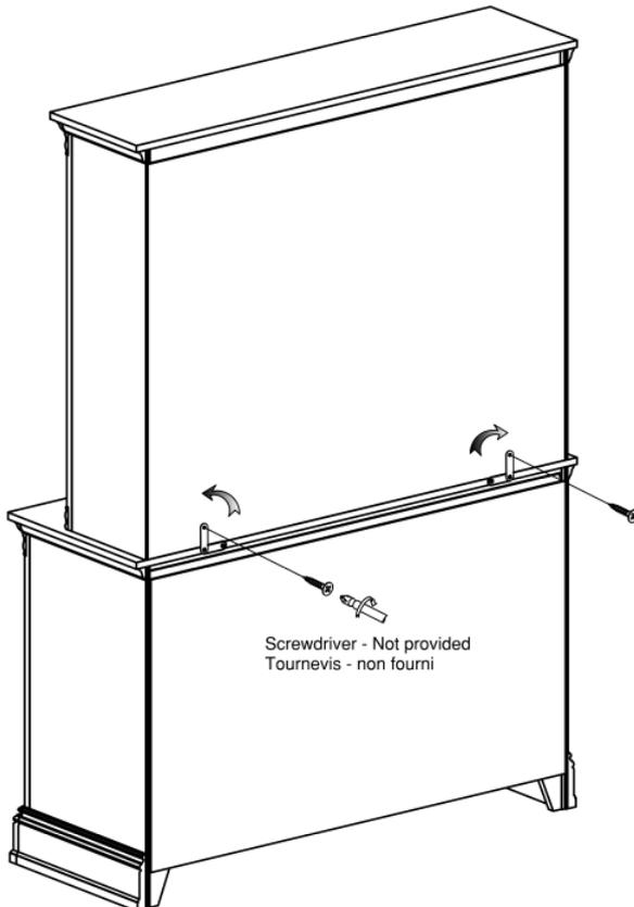
Turn the metal plate up and position into the hutch. Insert the same screw previously removed through the metal plate into the hutch with screwdriver (not provided).
