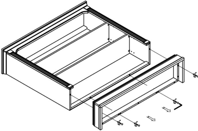
Remove the 4 bolts from the base with Allen wrench as shown. Keep the base and feet for future use.
