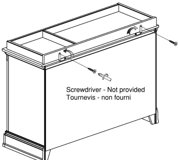
Turn the metal plate up and position into the changing tray. Insert the same screw previously removed through the metal plate into the changing tray with screwdriver (not provided).
